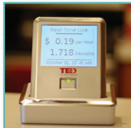
Advanced metering systems offer the consumer a gateway for tracking real-time power use and cost. Consumers can feed the information directly to home computers, if they prefer.
