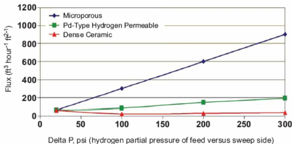
In addition to hydrogen partial pressure, other operating conditions such as temperature and quality of the feed stream can also influence hydrogen flux. Membrane attributes such as durability, cost, tolerance to contaminants, hydrogen recovery, and purity are also important factors in development of robust membranes that can be integrated into coal-based hydrogen production facilities.
