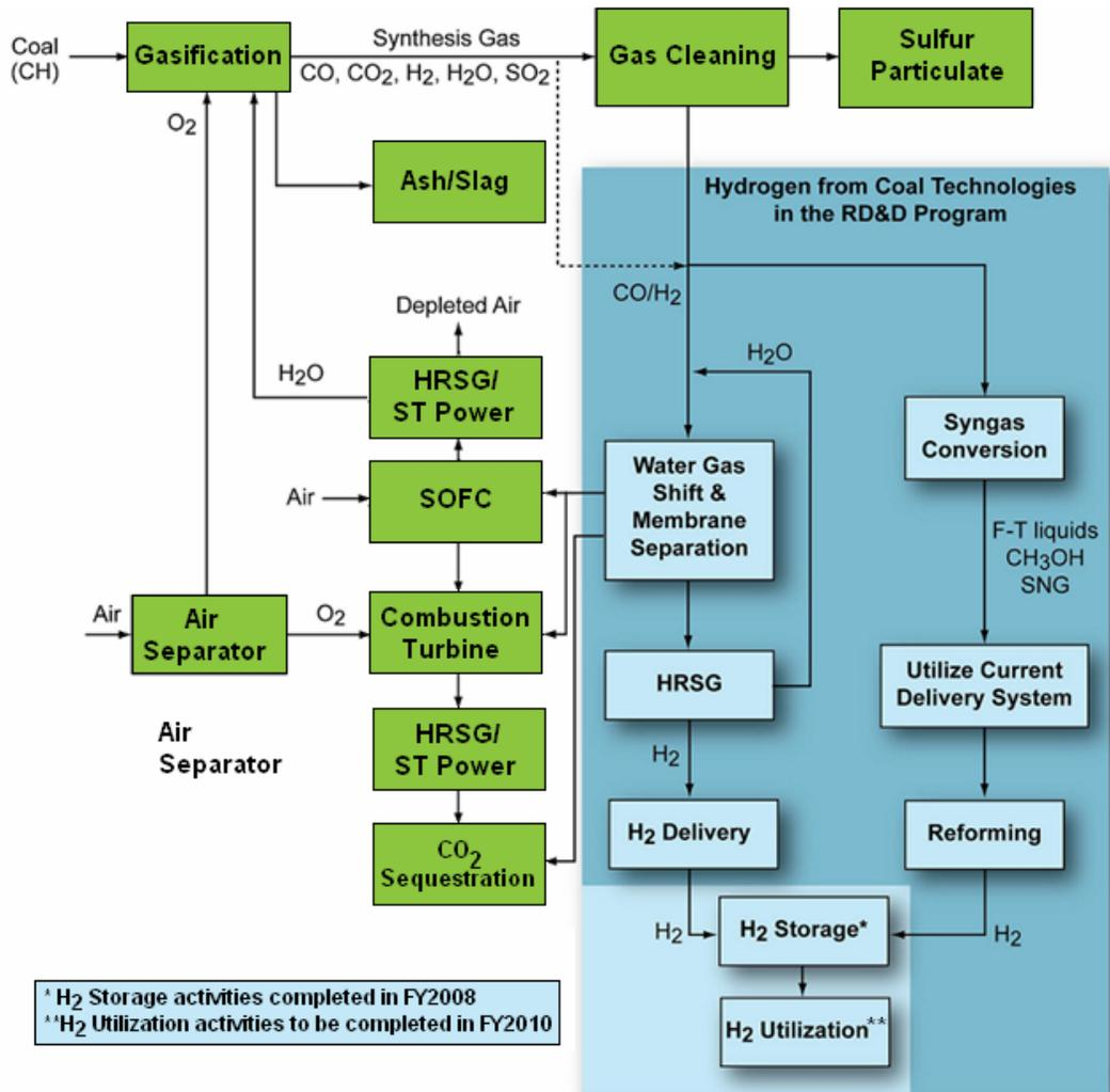
Figure 10. Key Elements of the Hydrogen from Coal Program
